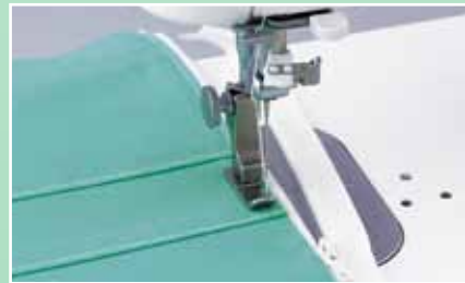
4 Hinged Cording Foot Suitable for edge sewing and overlapped seam
