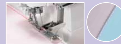
6 Beading Presser Foot For attaching pearls and beading with overlock stitching
