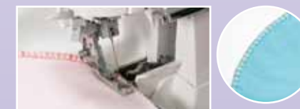
7 Curved Beading Presser Foot For attaching pearls and beading on a curve
