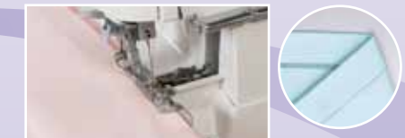
2 Blind Stitch Presser Foot (for Right Needle) For making blind hems
