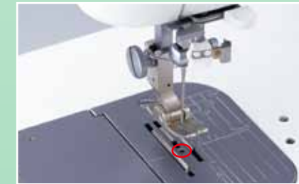
20 Throat Plate for Thick Fabric The large hole of throat plate is suitable for thick needle
