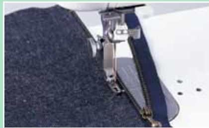
5 Hinged Zipper Foot Narrow width of foot feeds zipper smoothly
