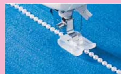
25 Pearl Attaching Presser Foot For attaching pearls, beads and thick cord
