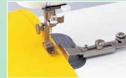
17 Swing Gauge To guide edge of fabrics (set by 2 screws)
