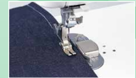
18 Magnetic Gauge To guide edge of fabrics
