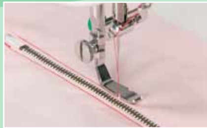
2 Zipper Attaching Foot Foot position can be moved to right or left
