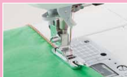
13 Hemming Presser Foot for Zigzag For hemming zigzag stitch with rolled fabric
