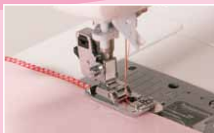
2 Overcasting Presser Foot It prevents the edge of fabric from fraying
