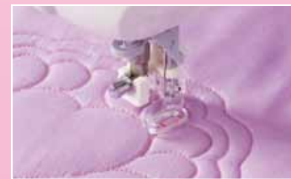
22 Quilt Presser Foot (transparent type) For free motion sewing and zigzag free motion sewing
