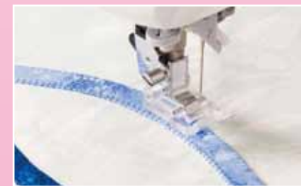
24 Applique Presser Foot For applique stitch (Front and back parts are short for easy movement at curve points)
