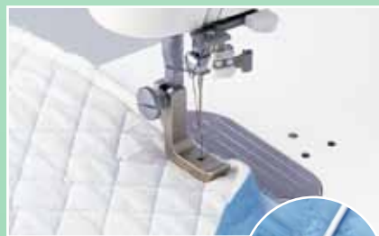
9 Piping Foot To attach corded piping
