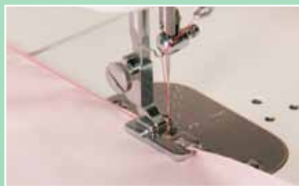
8 Hemming Foot For hemming stitch with rolled fabric (3mm)
