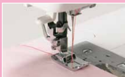
14 Straight Stitch Presser Foot For straight stitch sewing
