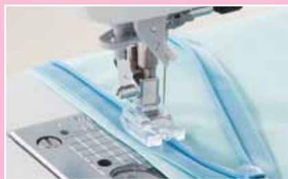
8 Invisible Zipper Foot For installation of concealed zipper
