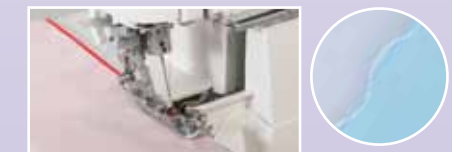
5 Cording Presser Foot For attaching nylon string or wire on edge of fabrics
